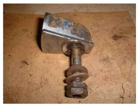
Remove the old silent block by using a bolt puller and continue turning until it becomes free. Then with a small screw driver remove the rubber "sleeve". Clean all faces. Use a piece of plastic tubing the diameter of the sleve with the aid of liquid soap, gently force tube and sleeve into base plate.
